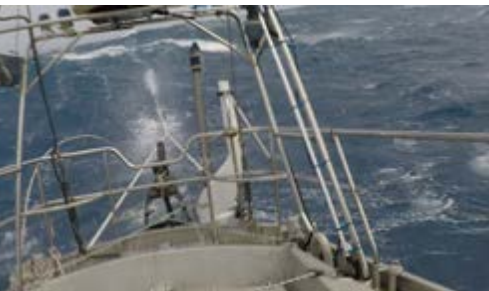
The Jordan Series Drogue (JSD) is deployed off the stern
