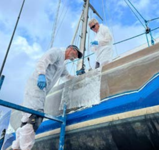
As it was just the two of us we used small sheets of glass that were more manageable
