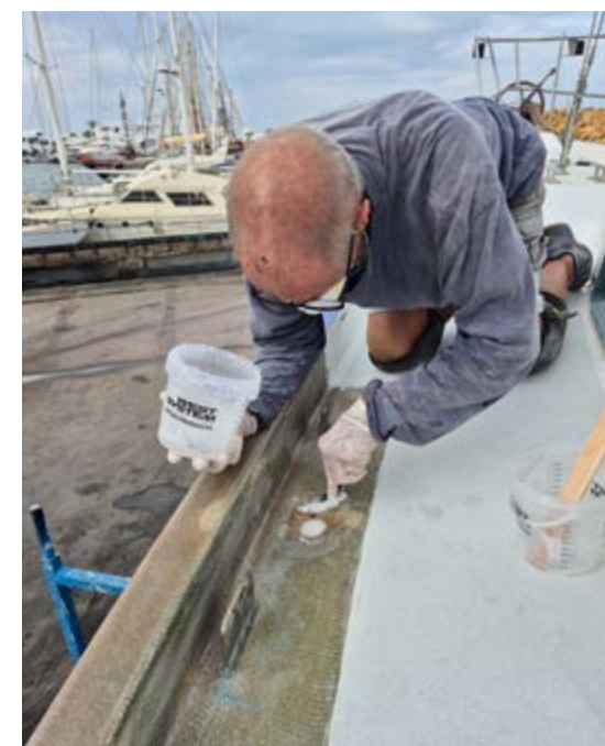
Clockwise from right: Lane filling the stanchion bolt holes with epoxy; cabinets removed revealing more repairs needed; even the port settee had to go to re-tab the bulkhead cracking along the inside of the bulwark
