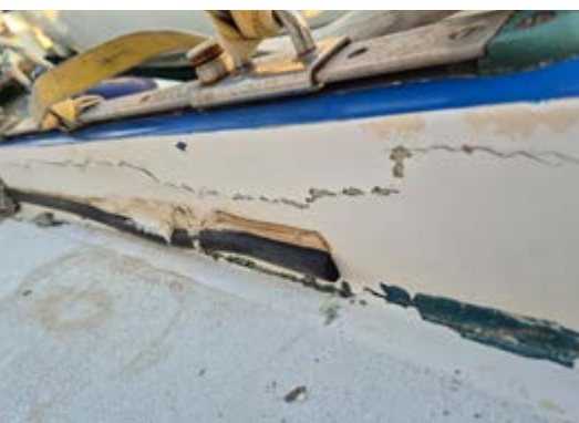
Clockwise from left: The 32mm x 6mm stainless jib track bent; ceiling panel inside the cabin cracked; cracking along the inside of the bulwark
