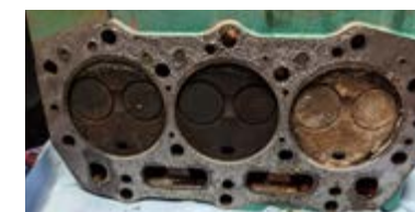
Salt and carbon had built up on the third piston before our time causing the engine to no longer turn over
